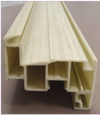
Fig. 5: A-PA6 composite profile for window application
